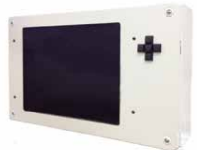
Monitor with protection box and crosshair generator
