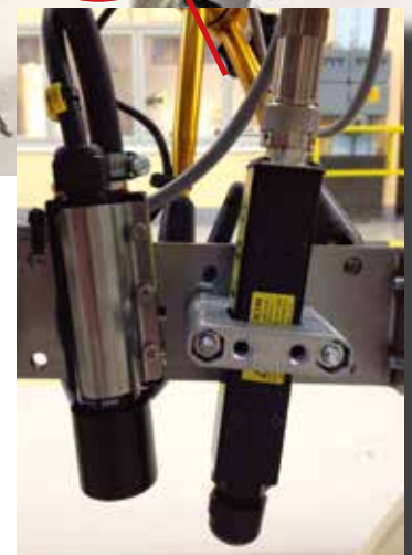
Camera installed onto bracket for welding torch
